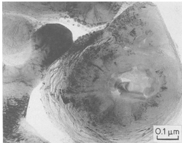
Figure 7 TEM image of spherulite showing concentric graphite growth and different core material.
